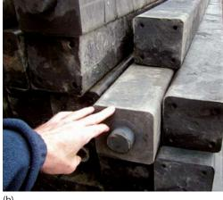
FIGURE 5 (a) A stack of downcycled railroad ties that were fabricated at the Berwick, Pa., plant, made from discarded geomembranes and (b) close-up of downcycled railroad ties at the Berwick facility (manufacturing by Axion International).
