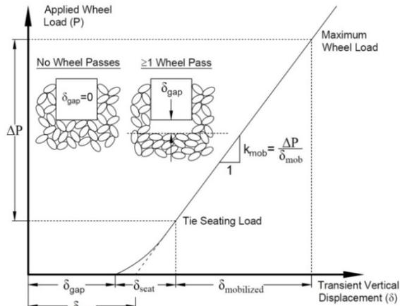
**FIGURE 4 – TRANSIENT VERTICAL DISPLACEMENT BEHAVIOR OF A TIE WITH GAP UNDER APPLIED WHEEL LOAD (GRAPH LOOKS BLURRY SO REPLACE WITH BETTER IMAGE????)**
