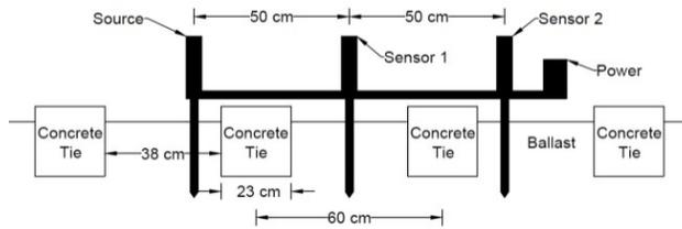
**FIGURE 9 – DIAGRAM OF FUTURE MODIFICATIONS TO BSPA DEVICE**
