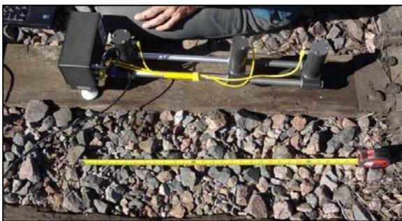
**FIGURE 3 – PHOTOGRAPH OF BSPA MEASURING MODULUS OF A TIMBER TIE**
