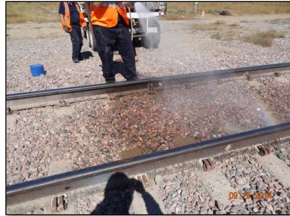
**FIGURE 5 – PHOTOGRAPH OF WETTING OF A SECTION OF CLEAN BALLAST**
