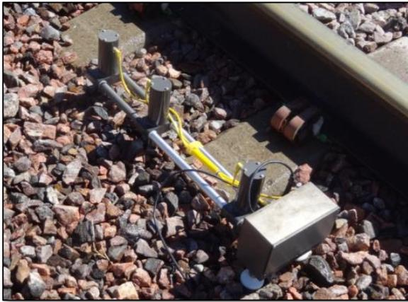
**FIGURE 2 – PHOTOGRAPH OF BSPA MEASURING BALLAST MODULUS UNDER A CONCRETE TIE**
