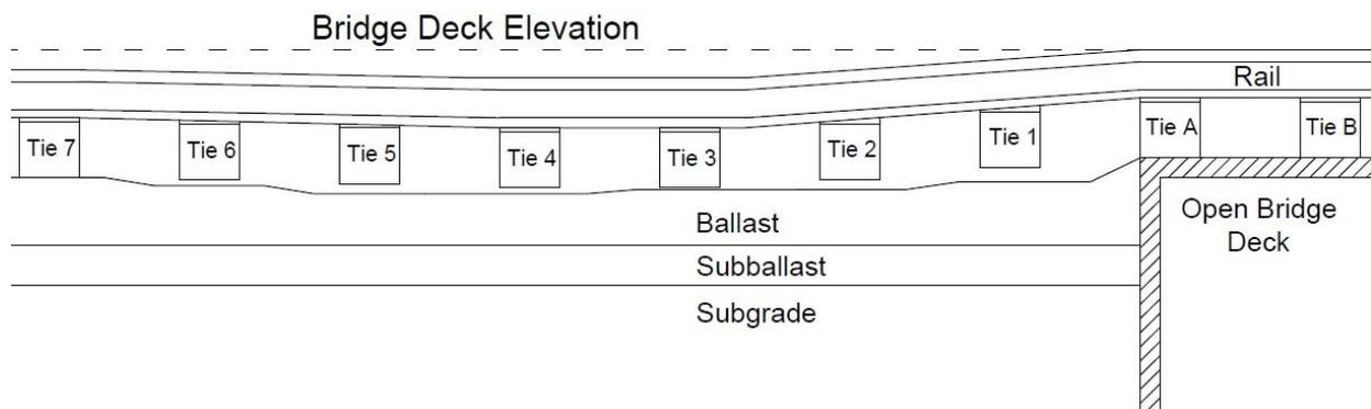
**Figure 1: Example diagrams of bridge transition zones with tie-ballast gaps.**
