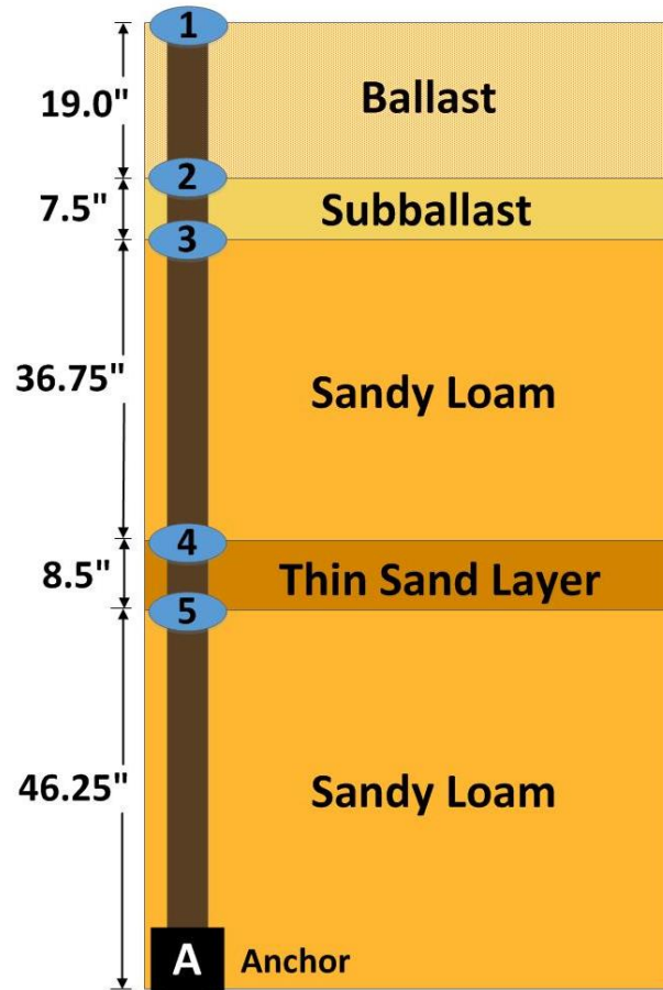
1 2 FIGURE 1 Subsurface profile and LVDT locations 60 feet north of Amtrak Upland 3 Street Bridge in Chester, Pennsylvania. 4 5
