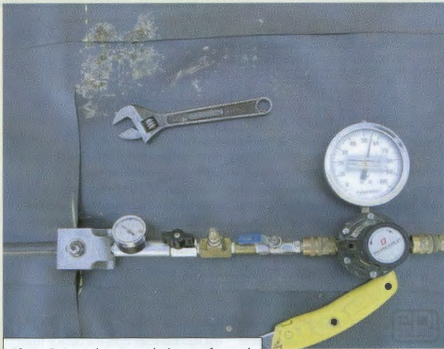
Photo 3. Seam burst test being performed.
