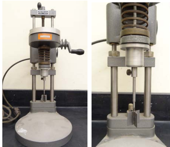
Figure 4: View of: (a) laboratory vane shear device and (b) close-up of laboratory vane.
