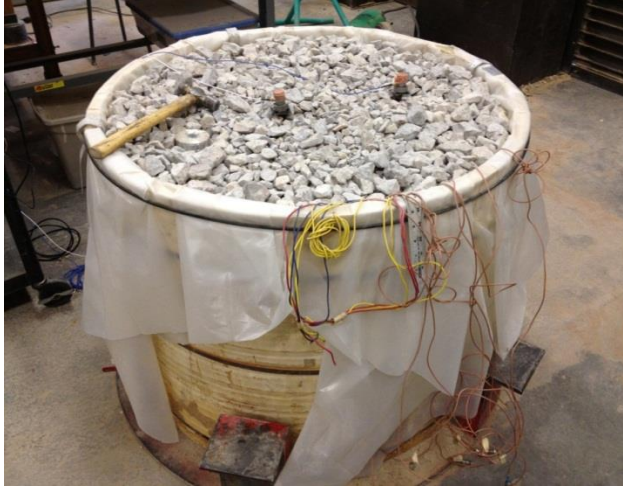
FIGURE 3 – GEOPHONE COUPLING CHAMBER AT UNIVERSITY OF TEXAS AT EL PASO
