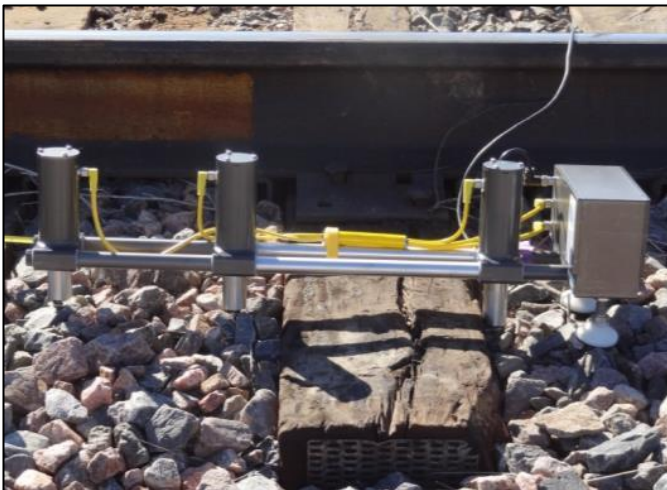
Figure 1: Photograph of BSPA measuring ballast modulus under the edge of a timber tie
