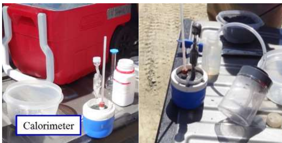
FIG. 5. Reactivity test performed at Subtitle D Landfill
