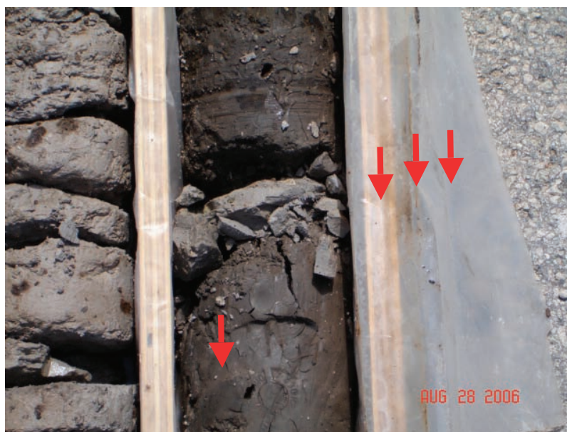
[FIG. 5] Grout fracture in the core for column S2-A1 at a depth of 23.8 m (78 feet) (arrows indicate grout found in the embankment materials)
