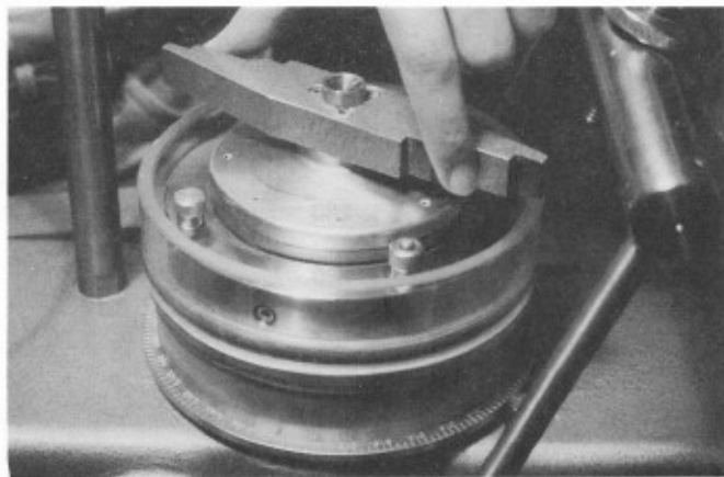
FIG. 4—Preshearing overconsolidated soil.
