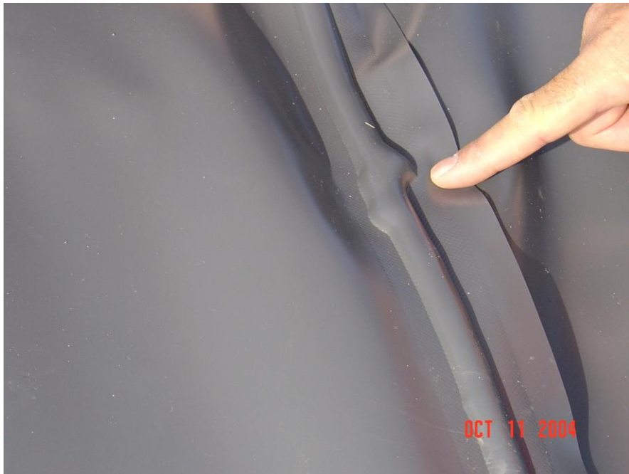
Figure 6. Aneurysm in 0.75 mm PVC geomembrane seam.
