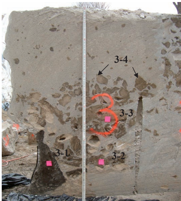
[FIG. 9] Soil inclusions and vertical hole from post-construction coring in triple fluid jet grout column #3.
