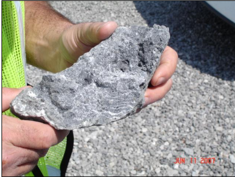
325 326 Figure 2: White dross excavated during gas well drilling in a Subtitle D landfill 327 experiencing an aluminum reaction 328
