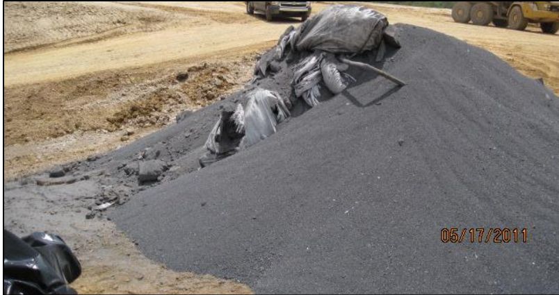
342 Figure 3: Pile of black dross disposed in APW monofill
