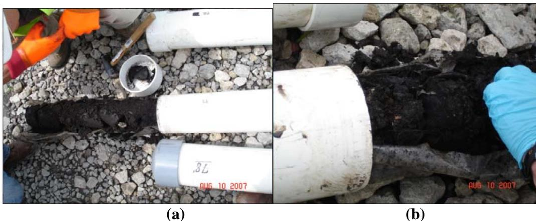
**Figure 3. Thermally degraded waste from 100 mm diameter sample**
