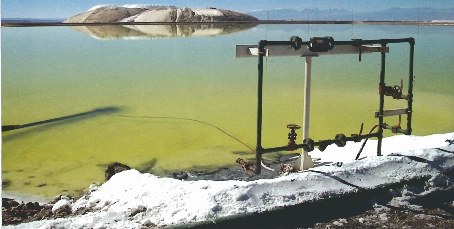
Photo 3 | A brine-filled evaporation pond at the Salar de Atacama in northern Chile. This photo shows one of the ponds filled with brine and undergoing evaporation. A pumping station in the brine-filled pond is shown in foreground. In the background are piles of extracted sodium chloride salt, with the Andes Mountains in the far background of this shot.
