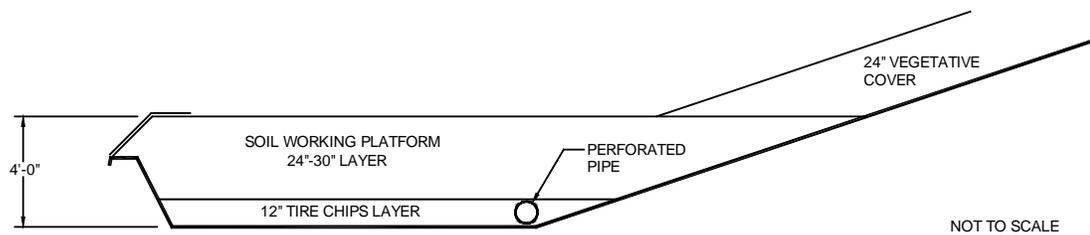
Figure 8: Remedial sideslope anchor detail
