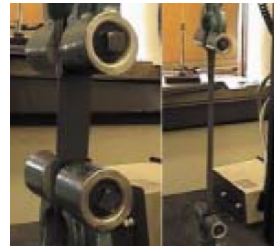
Photo 2: Exhumed PVC before and during tensile testing.
