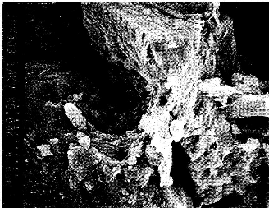
Fig. 1. Scanning electron microscope photograph of cementation joining two silt particles (magnification equals 500 times)
