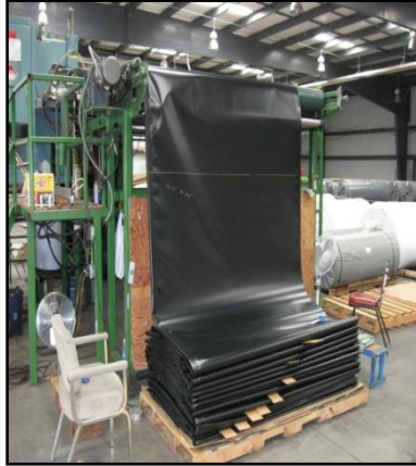
Figure 1 – Folding of 30 mil factory fabricated geomembrane panels
