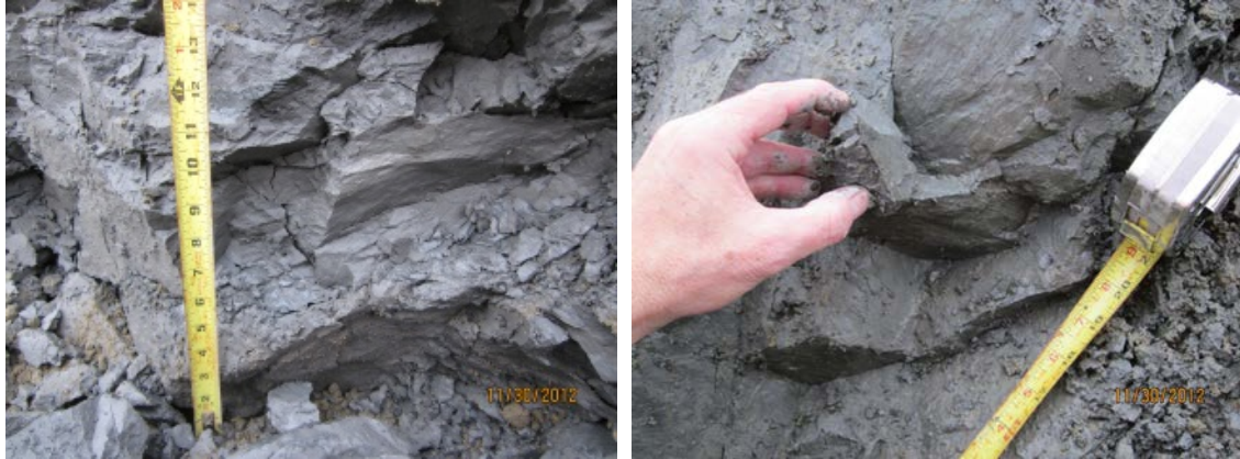
Figure 8. Photographs of highly jointed and fissured overconsolidated clay: (a) in shallow excavation and (b) close-up of joints and fissures and blocky nature of the overconsolidated clay.
