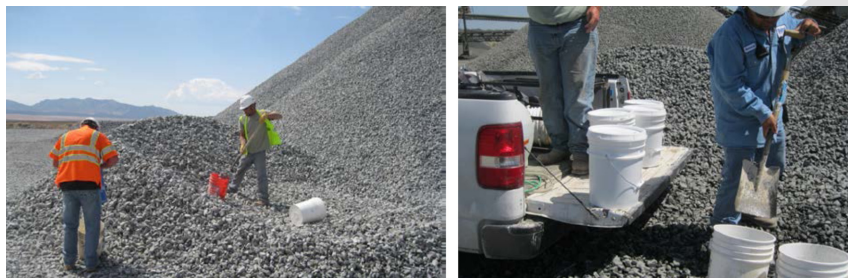
FIG. 2 Typical ballast stockpile sampling and filling buckets with stockpiled ballast (photos courtesy of Samuel C. Douglas).
