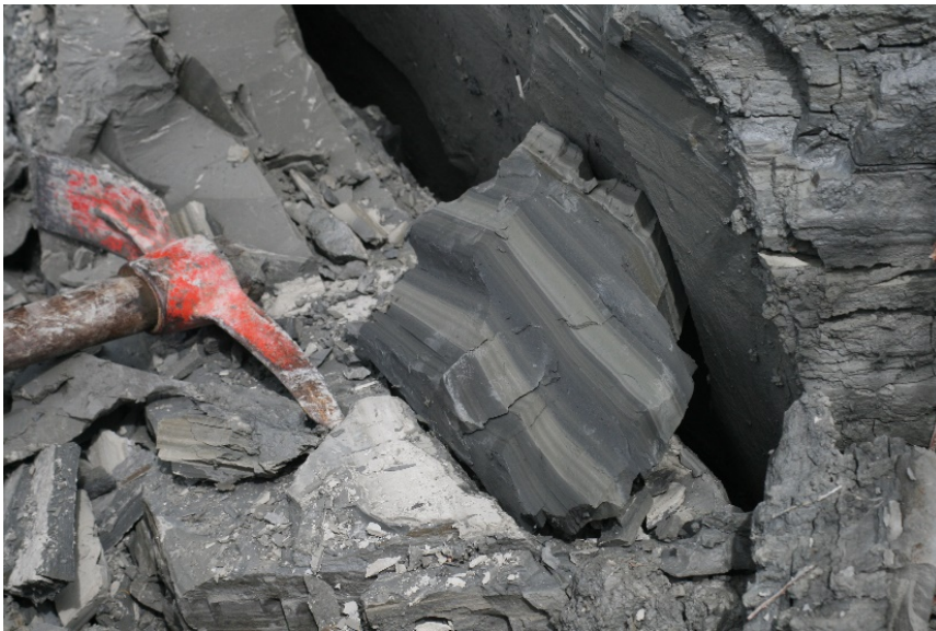
173 Figure 2: Unsaturated and overconsolidated glaciolacustrine silt and clay unit from 174 which the pre-existing colluvium was derived. Photo: J. Aaron.
