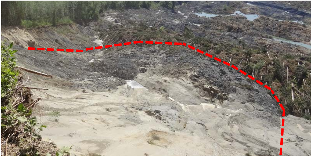
Figure 2: Close-up photograph on 22 May 2014 from headscarp of small debris avalanche cited by the Iverson Discussion (see dashed red line) as cause of second 22 March 2014 recorded ground motion. (Photograph by T.D. Stark; DSC09275.jpg)
