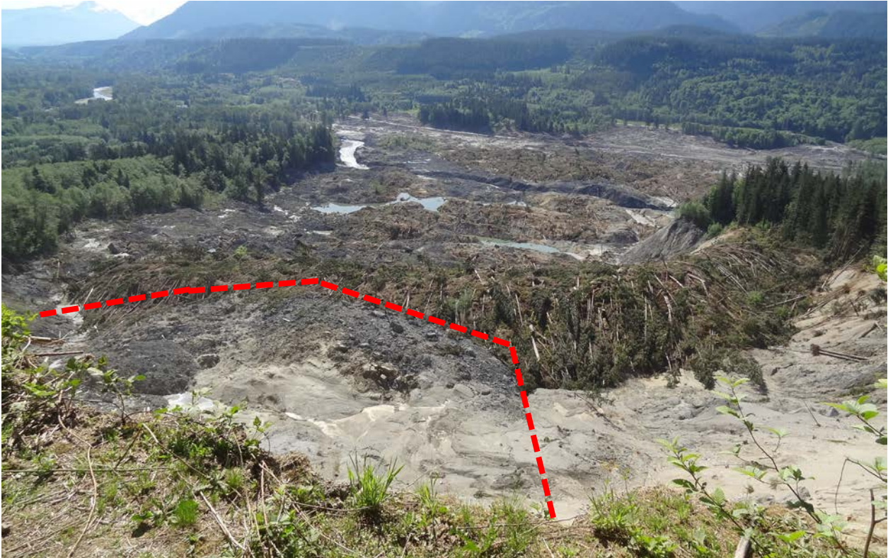
18 19 Figure 1: Photograph on 22 May 2014 from headscarp looking down on small debris 20 avalanche cited by the Iverson Discussion (see dashed red line) as cause of 21 second 22 March 2014 recorded ground motion. (Photograph by T.D. Stark; 22 DSC09275.jpg)
