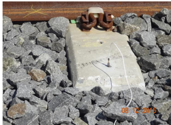
1 Figure 1: Upland Street northern Track #2 approach with UTPs: (a) diagram showing 2 instrumentation layout, (b) overview photograph of transition with orange 3 targets for video cameras, (c) Bending Beam with reference stake (see arrow) 4 located in crib, and (d) accelerometer attached to a concrete tie. 5
