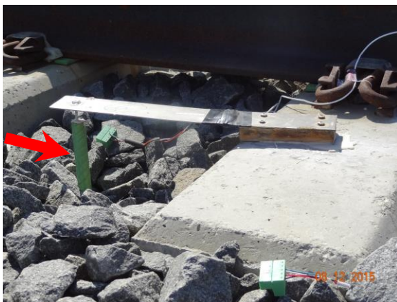
1 Figure 1: Upland Street northern Track #2 approach with UTPs: (a) diagram showing 2 instrumentation layout, (b) overview photograph of transition with orange 3 targets for video cameras, (c) Bending Beam with reference stake (see arrow) 4 located in crib, and (d) accelerometer attached to a concrete tie. 5
